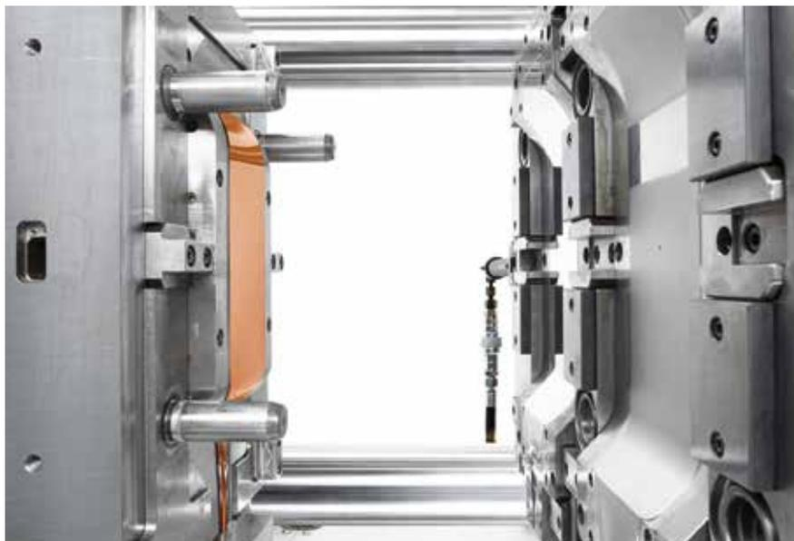
Almost ready-to-install parts can be withdrawn from the mold after flow-coating the injection-molded base body with a polyurea coating. The parts can even be multi-colored and can contain intricate logotypes, emblems or decorations
